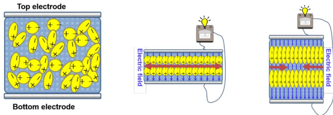
**Figure:** (a) A piezoelectric beam is an elastic beam with electrodes at their top and bottom surfaces, and connected to an external electric circuit. As voltage is applied to its electrodes, it actively (b) stretches or (c) shrinks in the longitudinal directions, therefore, causes charges to separate and line up in the vertical direction.
